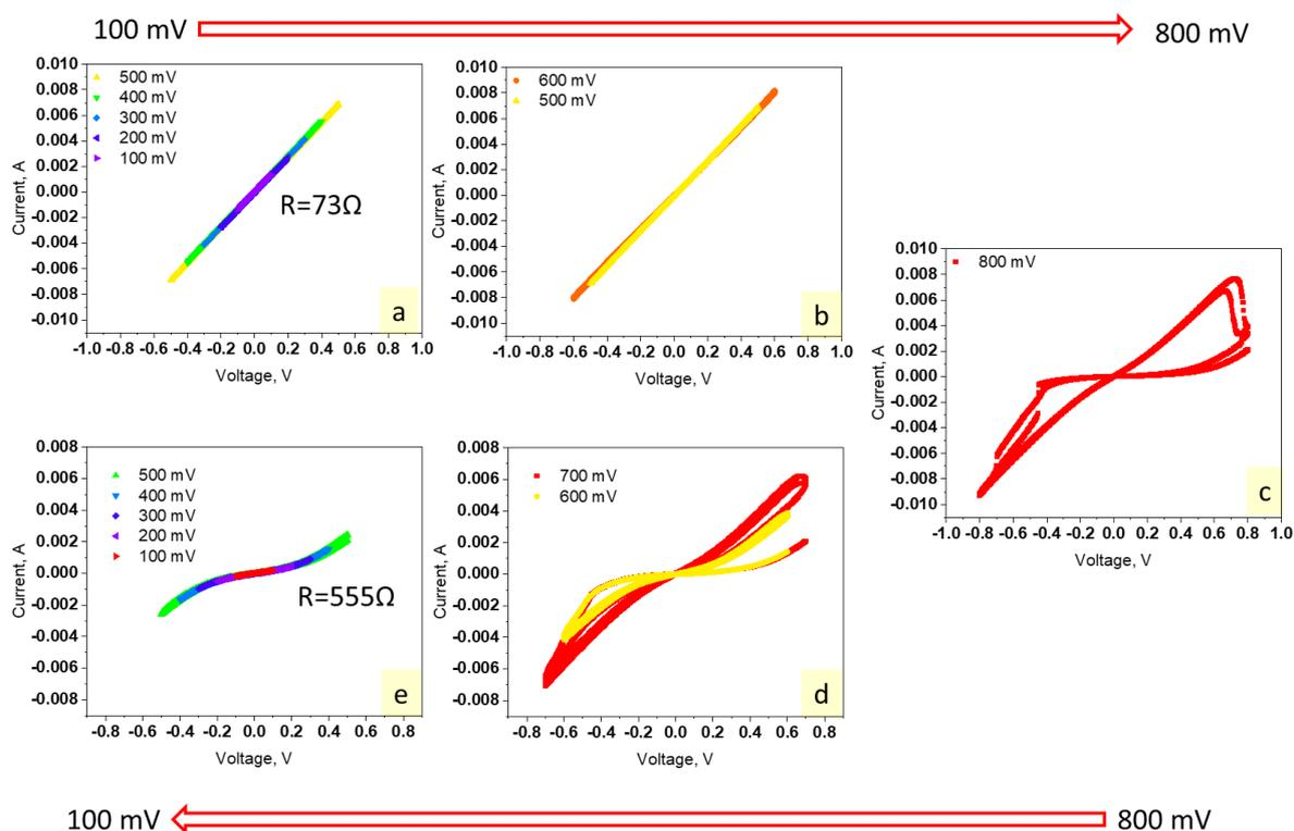
**Fig. A6:** I-V characteristics of a Ti/Au/BOC/Au/Ti device, demonstrating a) linear behavior from 100 to 500 mV, b) linear behavior with slight deviation at 500-600 mV and c) hysteresis loop at 800 mV, d) hysteric behavior at 700-600 mV, e) non-linear behavior from 500 to 100 mV.
