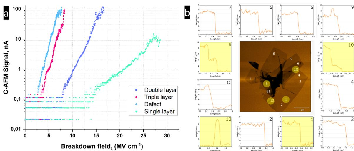
Fig. A1: a) C-AFM signal vs. breakdown field measured in four different zones corresponding to the 1<sup>st</sup>, 8<sup>th</sup>, 10<sup>th</sup> and 12<sup>th</sup> scans as shown in b) AFM scan of BOCN, with marked positions where height profiles are conducted; Scans 1 to 12: corresponding height profiles.
