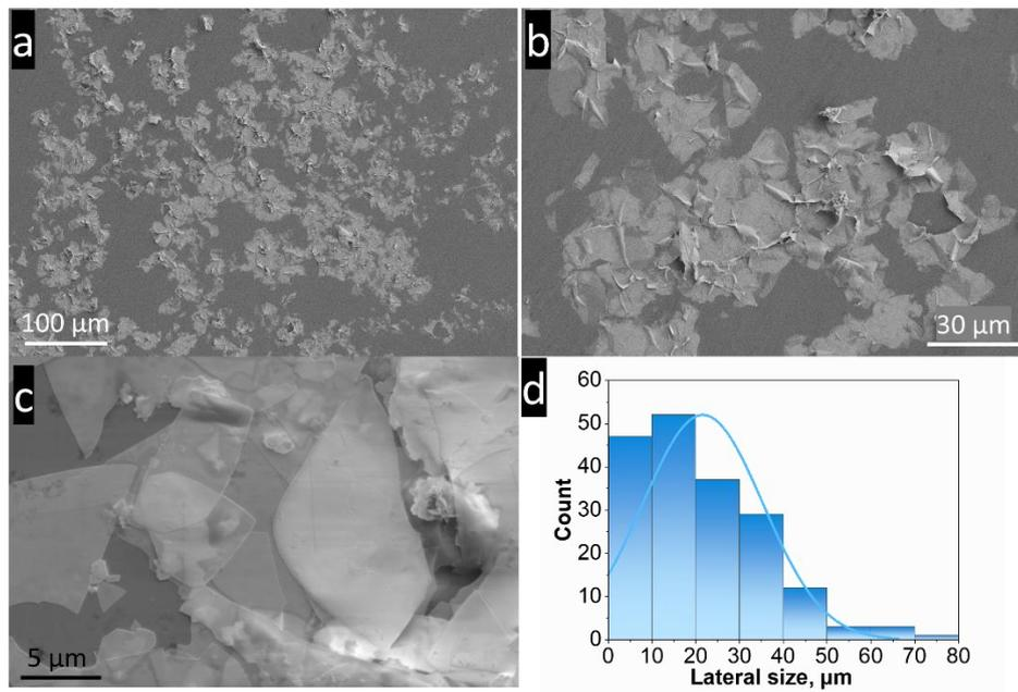
**Supplementary Material S3.1:** Low-magnification SEM images of a) nanosheets deposited on a Si substrate, b) magnified view of the nanosheets, c) magnified view of a bundle of nanosheets, d) lateral size distribution of synthesized nanosheets
