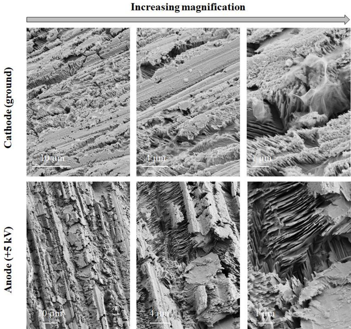
**Supplementary Material S2.7:** Comparison of the surfaces of anode and cathode after treatment in water. The same features (trenches and combs) are observed. Here again, nanosheets are only observed on the cathode, whichever the liquid.
