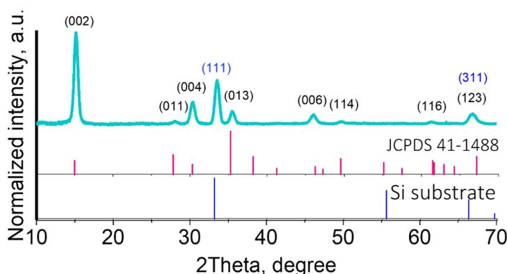
Fig. 3.12: XRD pattern of the nanosheet measured in Bragg-Brentano geometry. Comparison is made between the experimental pattern obtained with  $\lambda_{\text{Co}} = 1.78897 \text{ \AA}$  and the reference data from JCPDS 41-1488, corresponding to  $\text{Bi}_2\text{O}_2\text{CO}_3$  with the space group  $I4/mmm$ .
