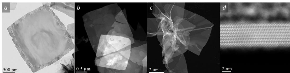
**Fig. 3.2:** **a)** BF TEM and **b-c)** HAADF STEM micrographs showing  $\text{Bi}_2\text{O}_2\text{CO}_3$  with most commonly encountered nanosheet morphologies, **d)** high resolution STEM FIB cross section micrograph of a BOC nanosheet along [100] zone axes.
