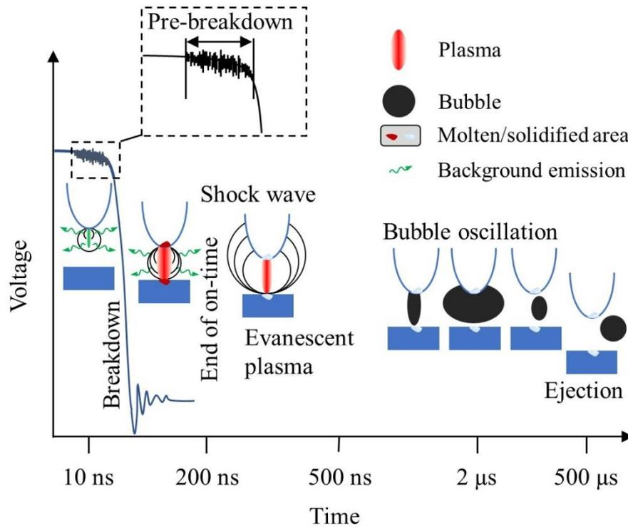
Fig. 1.3: Simplified sketch of events occurring in submerged discharge processes. After *J. Appl. Phys.* 113, 213303 (2013), with the permission of AIP Publishing (Fig. 1 in [Hamdan2013b]).
