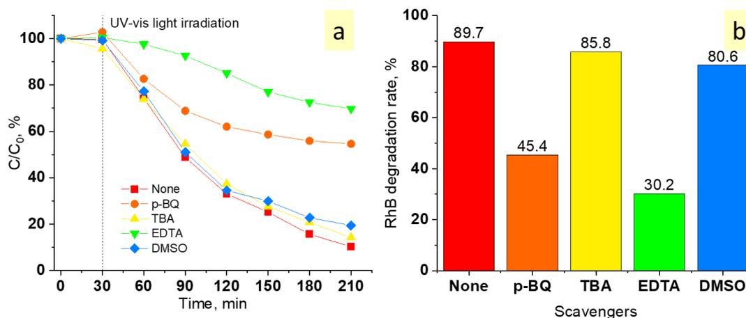
Fig. 4.5: Effects of radical scavengers on a) the RhB degradation using the Bi<sub>2</sub>O<sub>2</sub>CO<sub>3</sub> photocatalyst under UV-Vis light irradiation, b) conversion after 180 minutes of light exposure.
