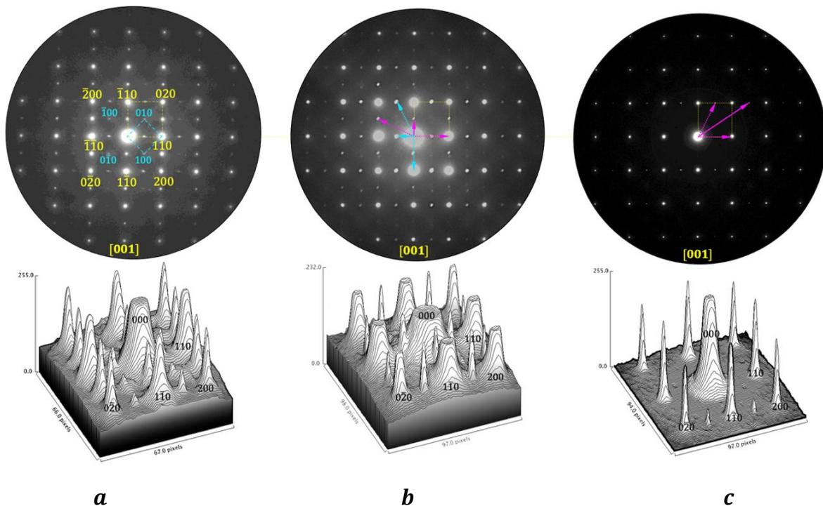
**Fig. 3.19:** Origin of the extra reflections on the electron diffraction pattern recorded along  $[001]$  on different area under the electron beam: **a)** order-disorder transformation (unit cell coloured in cyan), **b)** and **c)** multiple diffraction pointed out by vectors coloured in cyan and/or in magenta.
