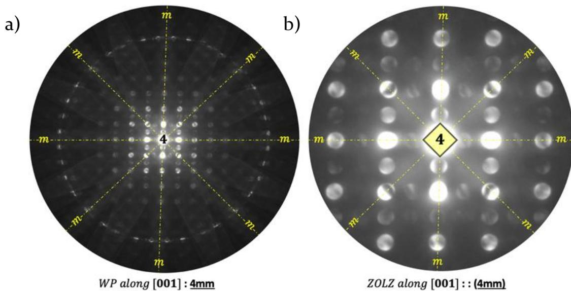
**Fig. 3.7:** Convergent beam electron diffraction (CBED) pattern recorded along  $[001]$  zone axis, **a)** the whole pattern ideal symmetry is  $4mm$ , **b)** the ZOLZ pattern ideal symmetry is also  $4mm$ .
