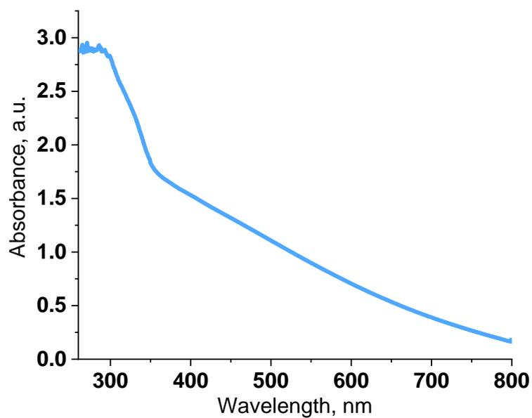
**Supplementary Material S4.3:** UV-Vis diffuse reflectance spectra (DRS) of Bi<sub>2</sub>O<sub>2</sub>CO<sub>3</sub>. The absorption peak is located at 360 nm, with a long tail extending beyond 800 nm. This tail is attributed to the scattering of nanoparticles present in the solution.
