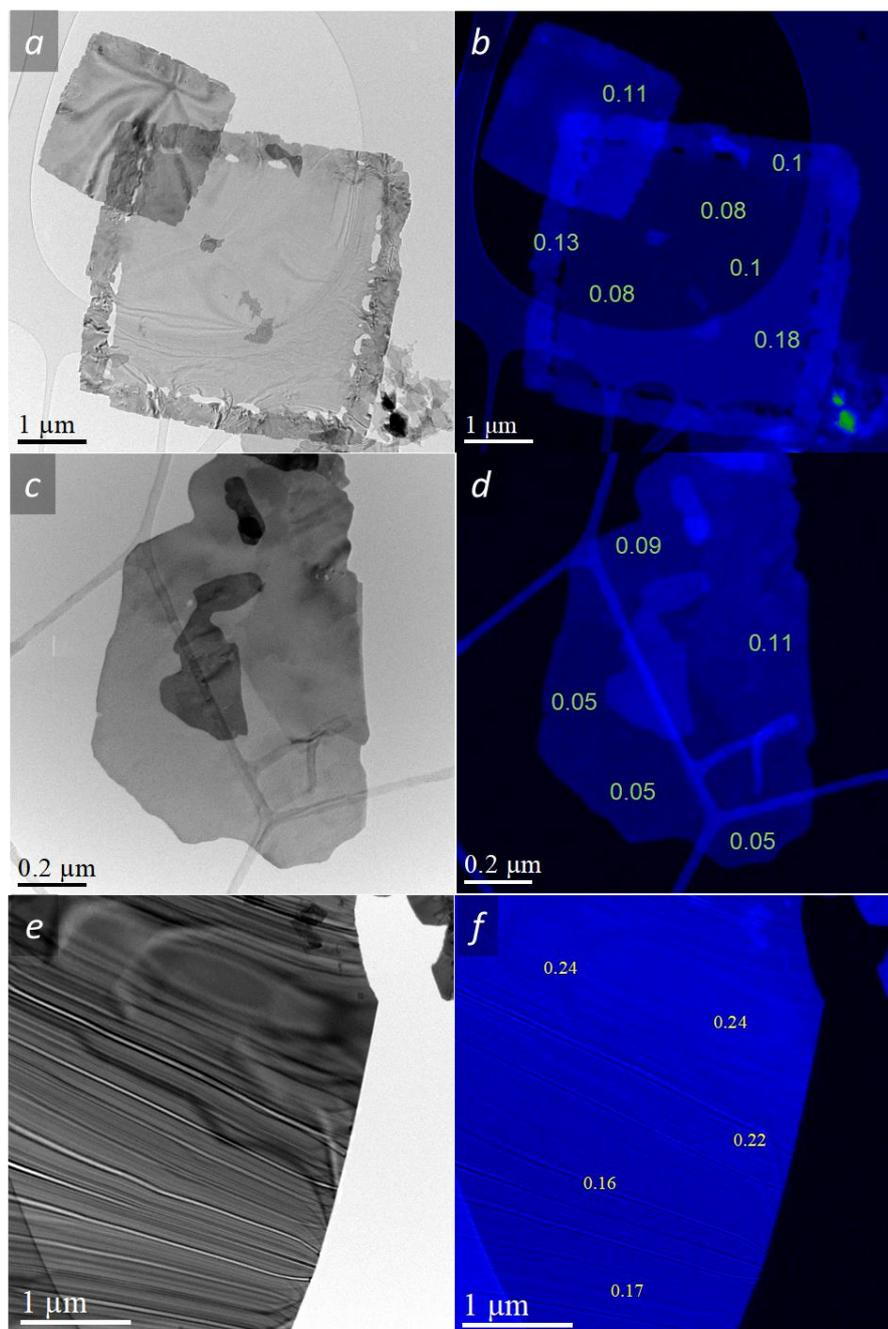
**Supplementary Material S3.2:** Examples of three nanosheets with different thicknesses: a,c,e) BF STEM micrograph of a BOC nanosheets deposited on a holey carbon TEM grid with b,d,f) corresponding EELS thickness mappings. Figs. 4a and 4c: examples of the thinnest nanosheets. Fig. 4e: example of the thickest nanosheet. These mappings indicate the values of the  $t/\lambda$  ratio needed for thickness estimation.
