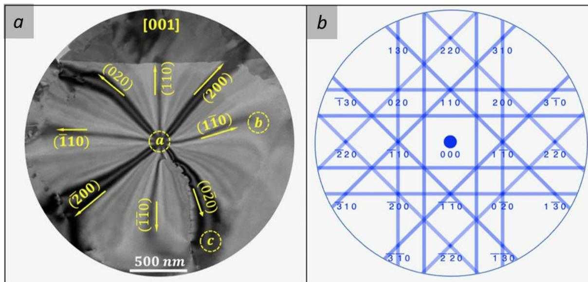
Fig. 3.18: a) BF-TEM micrograph recorded along  $[001]$  zone axis decorated by intersecting bend contours. The intersection of the bend contours can move from one area to another one (a, b or c) when the specimen under observation is slightly tilted. b) Diffraction pattern recorded along  $[001]$  zone axis and the corresponding Kikuchi bands diagram.
