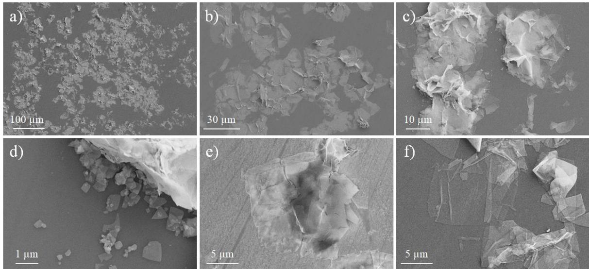
**Supplementary Material S2.1:** Scanning electron microscope (SEM) micrographs at different magnifications (**a**: x180, **b**:x700, **c**: x1400) of a silicon wafer covered in nanosheets (case of water but similar images are obtained with liquid nitrogen); **d**) small fragments around crumpled nanosheets; **e**) broken thick nanosheets; **f**) ultrathin nanosheets.
