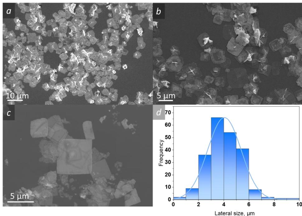
**Fig. 3.1:** Low-magnification SEM images of **a)** nanosheets deposited on a Si substrate, **b)** magnified view of the nanosheets, **c)** enlarged depiction of a squared sheet, **d)** lateral size distribution of synthesized nanosheets.
