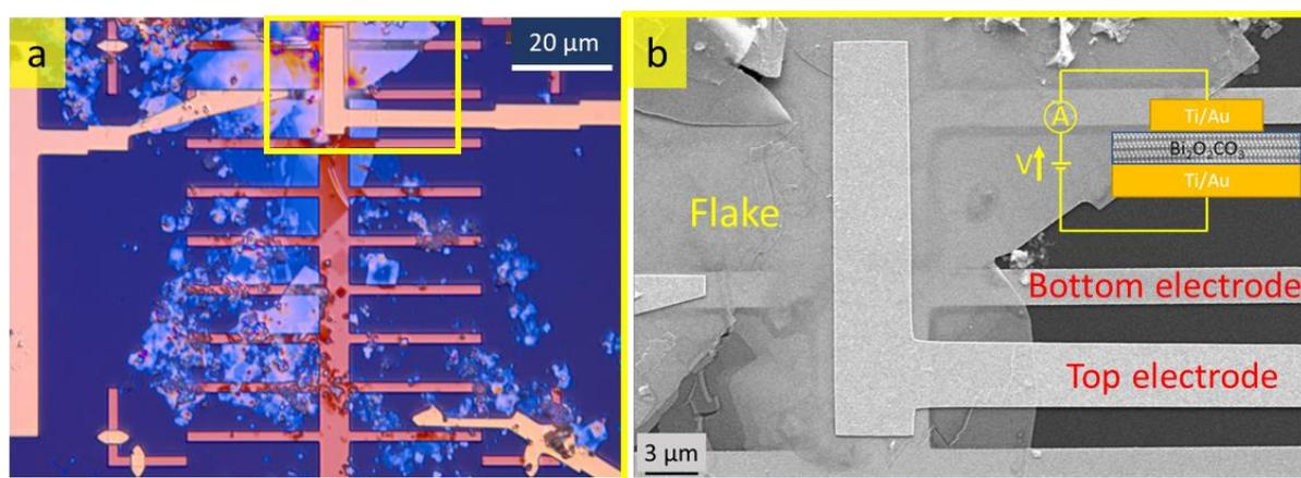
Fig. A5: The device structure. a) Optical image of the BOC based device on a Si/SiO<sub>2</sub> wafer, b) SEM micrograph of the yellow area of the device, insert shows the schematic diagram of the MIM type vertical BOC device.
