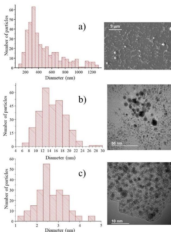
**Fig. 1.10:** Size distributions of particles produced by discharges in liquid. Three distributions are commonly found. The two lowest distributions can overlap, leading to two main distributions, as it is described in some other processes like pulsed laser ablation in liquid. *Reproduced with permission from Elsevier – Materials Chemistry and Physics* (Fig. 4 in [Hamdan2013d]).
