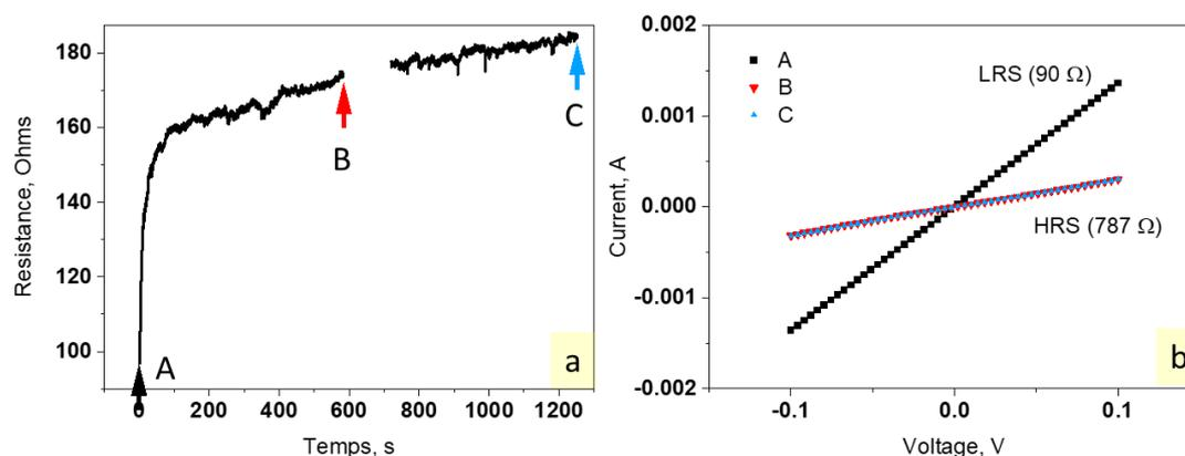
Fig. A8: a) Time evolution of resistance measured with a polarization voltage  $+800\text{ mV}$  after 20 min of resetting at  $V$  reset of  $-800\text{ mV}$ , b) IV log curves ( $V_{\max}=100\text{ mV}$ ) taken at the time A, B and C indicated in a)
