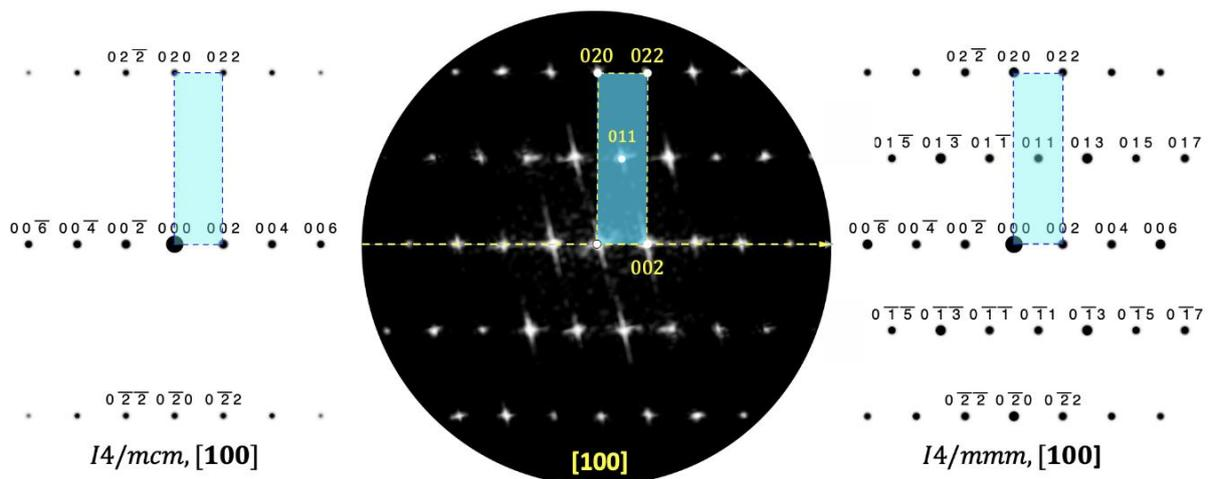
Fig. 3.10: Parallel between the simulations of the diffraction patterns of the space groups  $I4/mcm$  and  $I4/mmm$  obtained along the zone axis  $[100]$  and the FFT of the HREM image of the BOC nanosheet recorded along the same zone axis  $[100]$ . We can point out the similarity between the simulation corresponding to the space group  $I4/mmm$ , and the FFT of the experimental HREM of the BOC nanosheet obtained along the same zone axis  $[100]$ .
