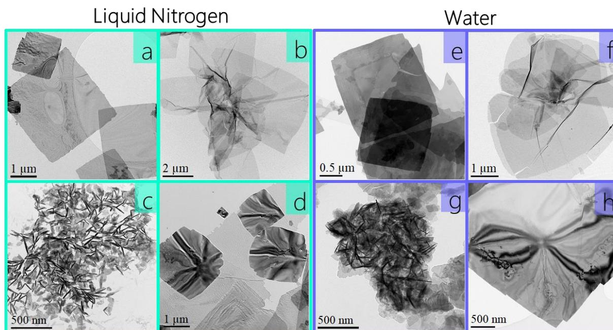
**Fig. 2.2:** Bright Field TEM micrographs showing the different shapes of nanosheets synthesized in liquid nitrogen and in water. **a)** and **e)** thin flat nanosheets. **b)** and **f)** thin crumpled nanosheets. **c)** and **g)** thin rolled nanosheets. **d)** and **h)** thick flat nanosheets.
