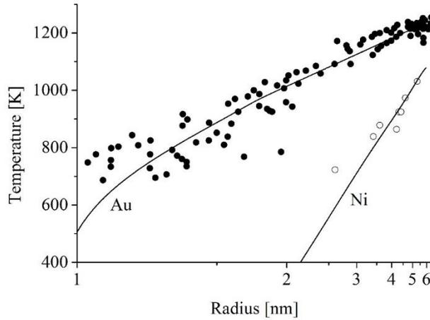
**Fig. 1.7:** Experimental data and Gibbs-Thomson curves established from Eq. (1) showing the size dependence of the melting temperature of gold [Font2013] and nickel [Teijlingen2020] nanoparticles in an  $(Y - 1/X)$  graph. The behaviour is almost linear beyond 2 nm in this graph and follows a reciprocal law.
