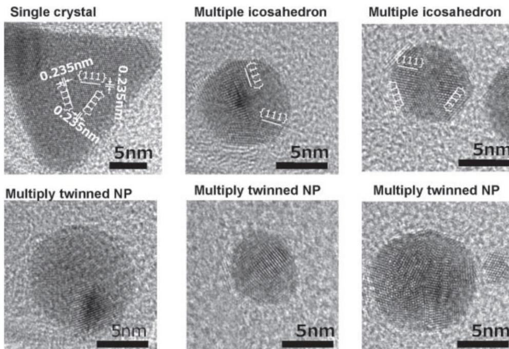
**Fig. 1.6:** HRTEM micrographs of gold nanoparticles synthesized by discharges in reverse micelle solution. The synthesized gold nanoparticles have different crystal features like fcc single-crystalline particles, multiply twinned particles, and incomplete multiply twinned particles (single-nanotwinned fcc configuration). Reproduced with permission from IOP Science – Japanese Journal of Applied Physics (Fig. 7 in [Saito2018]).
