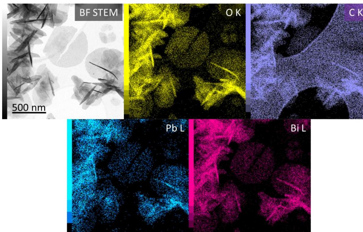
**Fig. 5.1:** BF STEM image of  $\text{Bi}_2\text{O}_2\text{CO}_3$  nanosheet and elemental mapping measurements showing the distribution profiles of Bi (magenta), Pb (cyan), O (yellow), and C (purple) elements.
