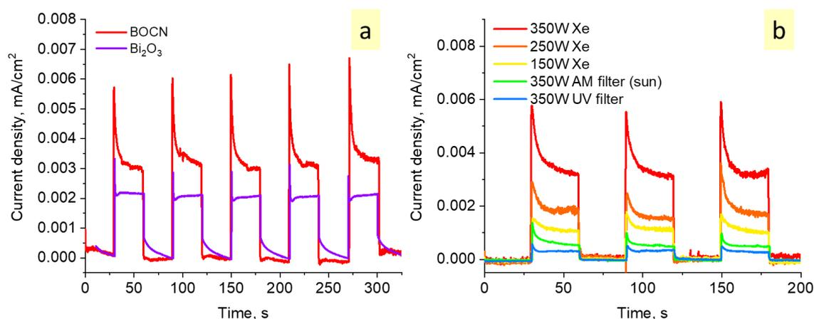
**Fig. 4.3:** a) Transient photocurrent response (0.15 V vs Ag/AgCl) of BOCN and commercial  $\text{Bi}_2\text{O}_3$  under UV-visible illumination (Xe lamp at 350 W), b) photocurrent density of BOCN at 0.15 V vs Ag/AgCl as a function of the light source
