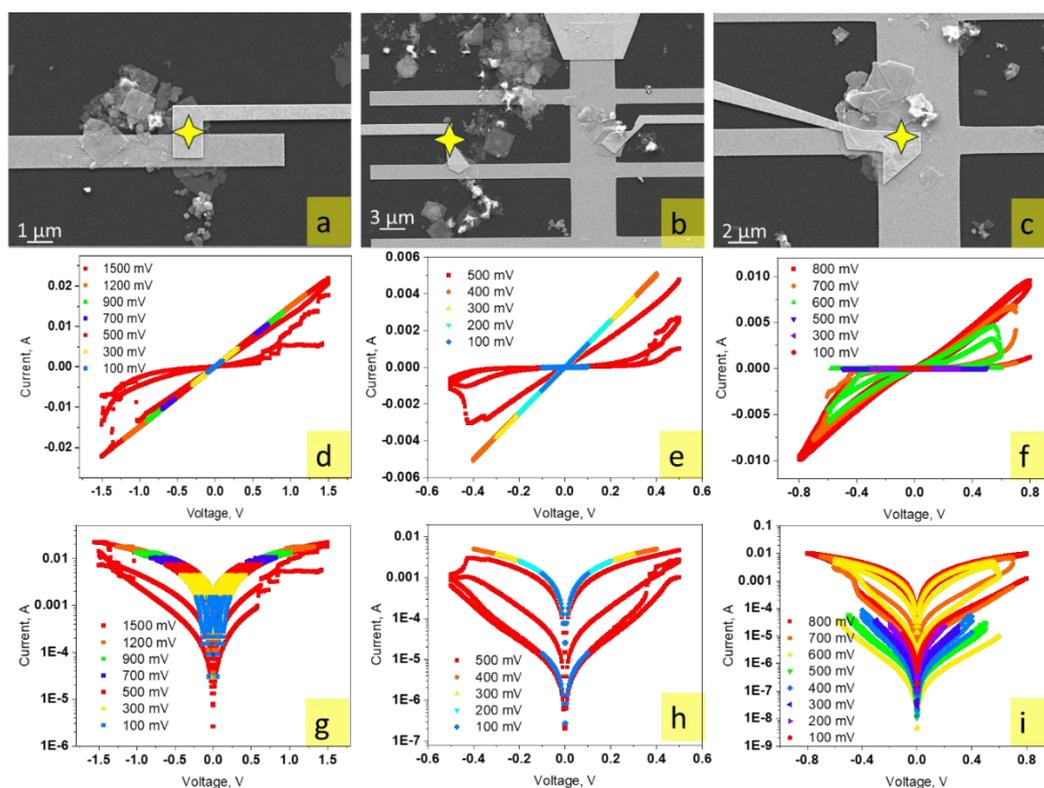
**Fig. 9:** a,b,c) SEM images of a three different Ti/Au/BOC/Au/Ti devices with d,e,f) their corresponding IV curves and log scale curves g,h,i).
