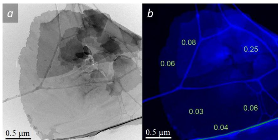
**Fig. 3.4:** Example of the thin nanosheet a) BF STEM micrograph of a BOC nanosheet deposited on a holey carbon TEM grid with b) corresponding EELS thickness mapping. These mappings indicate the values of the  $t/\lambda$  ratio needed for thickness estimation.
