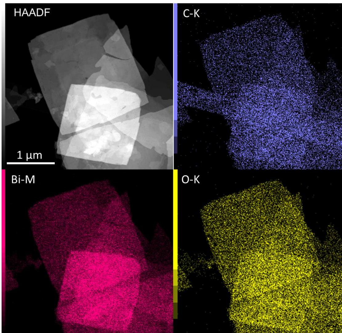
Supplementary Material S3.4: The STEM HAADF micrograph of a  $\text{Bi}_2\text{O}_2\text{CO}_3$  nanosheet and corresponding EDS elemental mapping of C, Bi and O respectively
