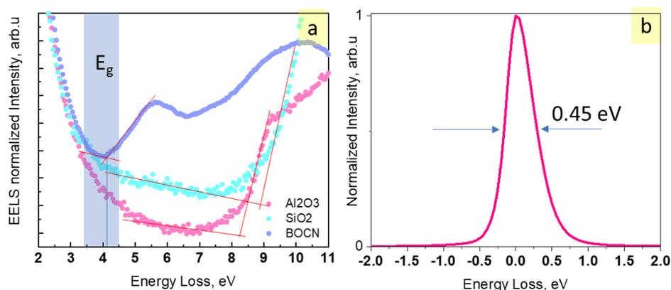
**Fig. A2:** a) STEM-EELS spectra (valence band excitations) collected with primary electron beam of 200 keV for BOCN, Al<sub>2</sub>O<sub>3</sub> and SiO<sub>2</sub> with applied linear-fit method used to calculate a bandgap energy of ~ 4 eV for BOCN, compared to ~ 8 eV for Al<sub>2</sub>O<sub>3</sub> and ~ 9 eV for SiO<sub>2</sub>. b) Zero loss peak acquired from JEM - ARM 200F Cold FEG. Normalized intensity is shown on a linear scale. The full-widths at half-maximum is 0.45 eV.
