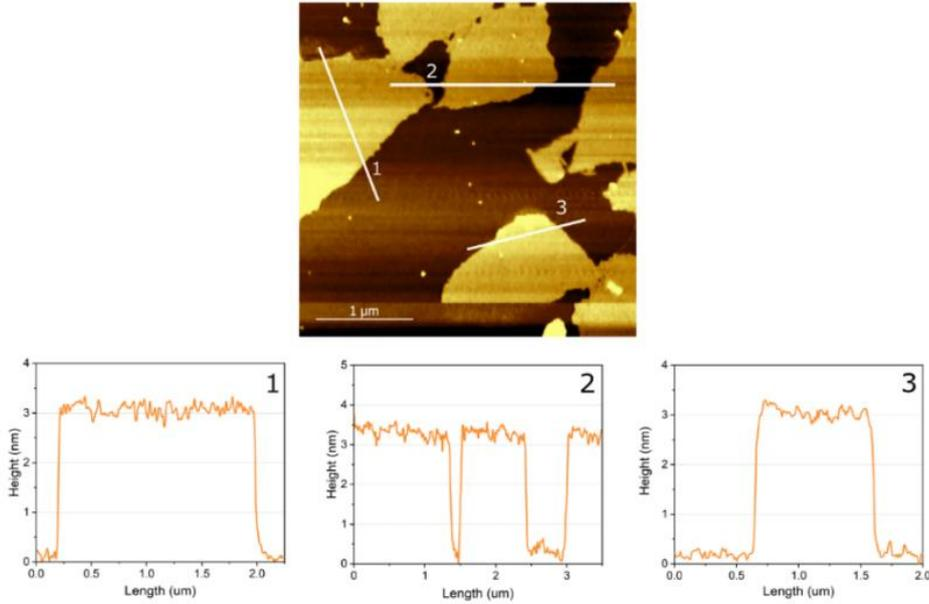
**Fig. 3.3:** AFM height-sensor micrograph depicting an individual BOC nanosheet. This micrograph provides a one-dimensional step height profile along the white lines labeled as 1-3. Corresponding cross-sections accompany these profiles, offering additional visual information.
