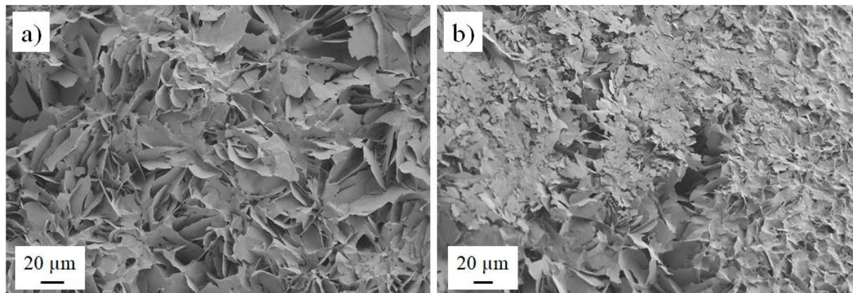
**Fig. 2.4:**  $\text{Bi}_2\text{O}_2\text{CO}_3$  nanosheets formed in the air after 6 days. a) Detail of the basal nanosheets. b) SEM micrograph showing two trenches and nanosheets covering the gap between them.
