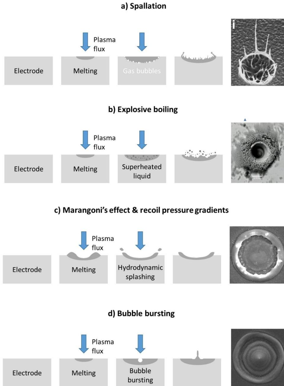
**Fig. 1.4:** Typical shapes of impacts and related underlying mechanisms leading to the production of large particles. Pictures in **a)** and **b)** are reproduced with permission from Elsevier – *Physics Procedia* (Fig. 1 in [Kuchmizhak2017]) and from Elsevier – *Materials Research Bulletin* (Fig. 4 in [Knotek2013]). Other pictures are current authors' credits. All spot sizes are around 10-20  $\mu\text{m}$  in diameter.
