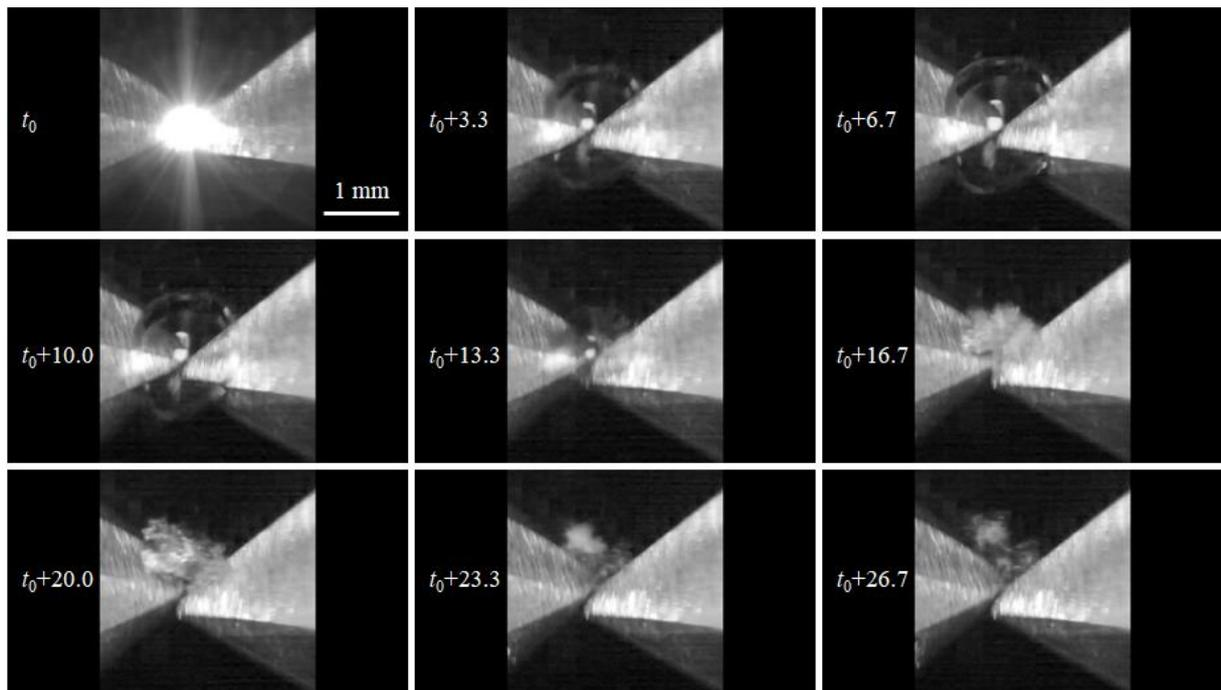
**Supplementary Material S2.9:** Set of pictures showing the transfer of nanosheets by mechanical sweeping of the surface by the bubble-liquid interface. The time scale is in  $\mu\text{s}$ . Discharge conditions are those reported in the experimental part. This event is characterized by the fact that the bubble expands and collapses one time only.
