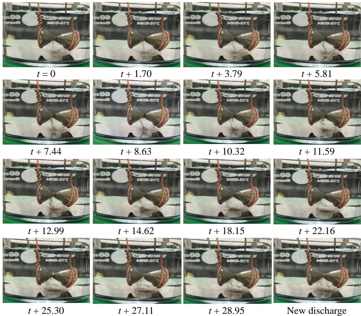
Supplementary Material S2.8: Set of pictures showing the movement of the generated particles in the liquid between two discharges. The time scale is in second. Particles remain at the bottom of the beaker, settling by gravity.
