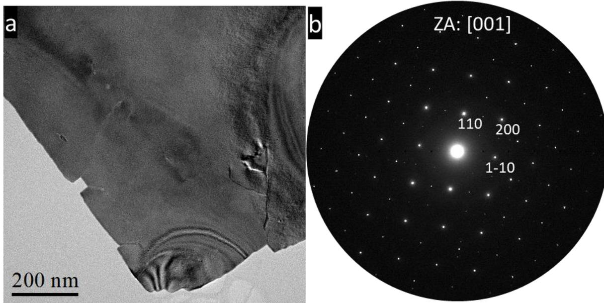
Supplementary Material S4.2: a) BF TEM micrograph of  $\text{Bi}_2\text{O}_2\text{CO}_3$  nanosheet with b) corresponding SAED pattern indexed as tetragonal phase  $\text{Bi}_2\text{O}_2\text{CO}_3$  PDF file 41-1488 in  $[001]$  zone axis
