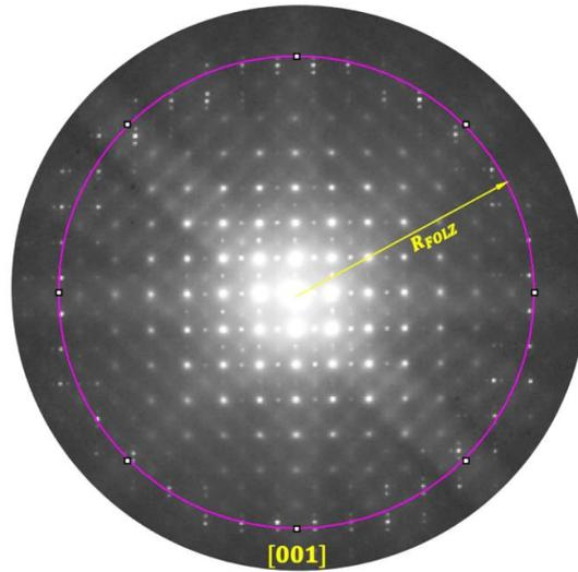
**Fig. 3.6:** Experimental diffraction pattern recorded along  $\langle 001 \rangle$  for the cubic system or  $[001]$  for the tetragonal system pointing out the  $R_{FOLZ}$ , the radius of the FOLZ. The latter is related to the range parameter  $P_{\langle 001 \rangle}$  ( $P_{\langle 001 \rangle}$  for the cubic system or  $P_{[001]}$  for the tetragonal system)
