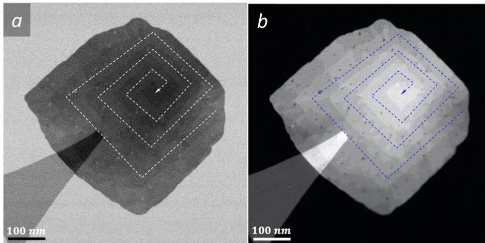
**Fig. 3.17:** a) TEM-Bright Field micrograph showing the BOC nanosheet developed by jog (terrace  $// [001]$  and front  $// [001]$ ) effect reminiscent of a spiral development. b) Corresponding TEM-Dark field. The dashed lines point out the spiral effect.
