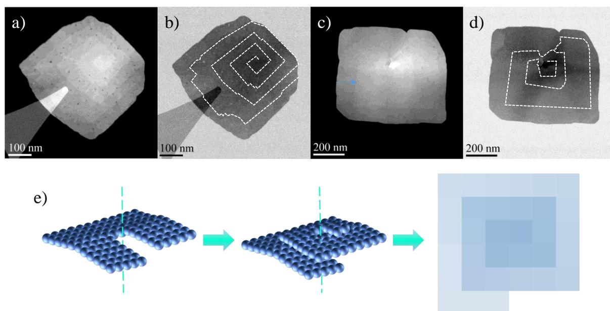
**Fig. 2.8:** a) and b): bright field and dark field STEM images of a nanopyramid. c) and d): another example. Dotted lines reproduce the spiralling edge of the pyramid. e) 3D view of steps leading to 3D-growth.
