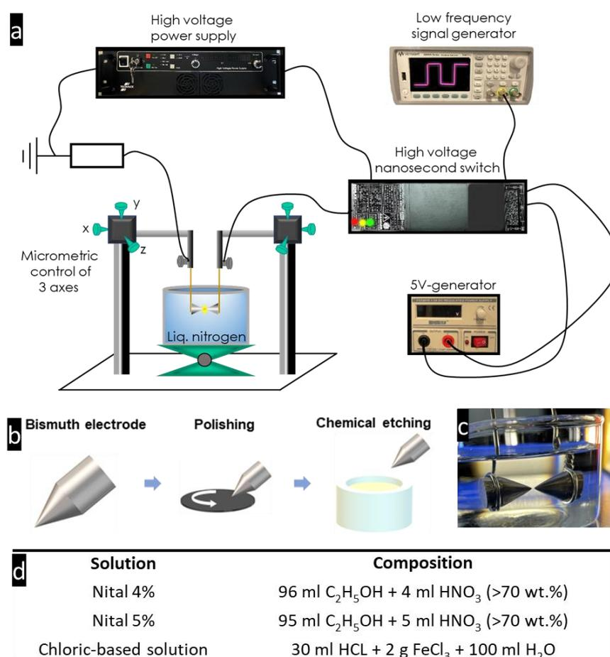
**Fig. 2.1:** a) Schematic of the experimental setup, here presented in the case of liquid nitrogen. b) Pre-treatment of the electrodes leading to a cone-shaped pin etched in one of the chemical solution presented in d). c) Picture of the electrodes in milli-Q water. d) Composition of the four chemical solutions tested in this work.
