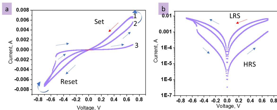
**Fig. A7**: Characteristic  $I-V$  curves of the MIM device based on a BOC material at  $V_{\max}$  700 mV. a) and b) show the typical  $I-V$  curves of the device; the original curves in a) represent a 2 cycle switching process (1<sup>st</sup> cycle loop depicted 1-2, 2<sup>nd</sup> cycle loop 2-3) and a log scale curves in b) show obvious low and high resistance states (LRS and HRS).
