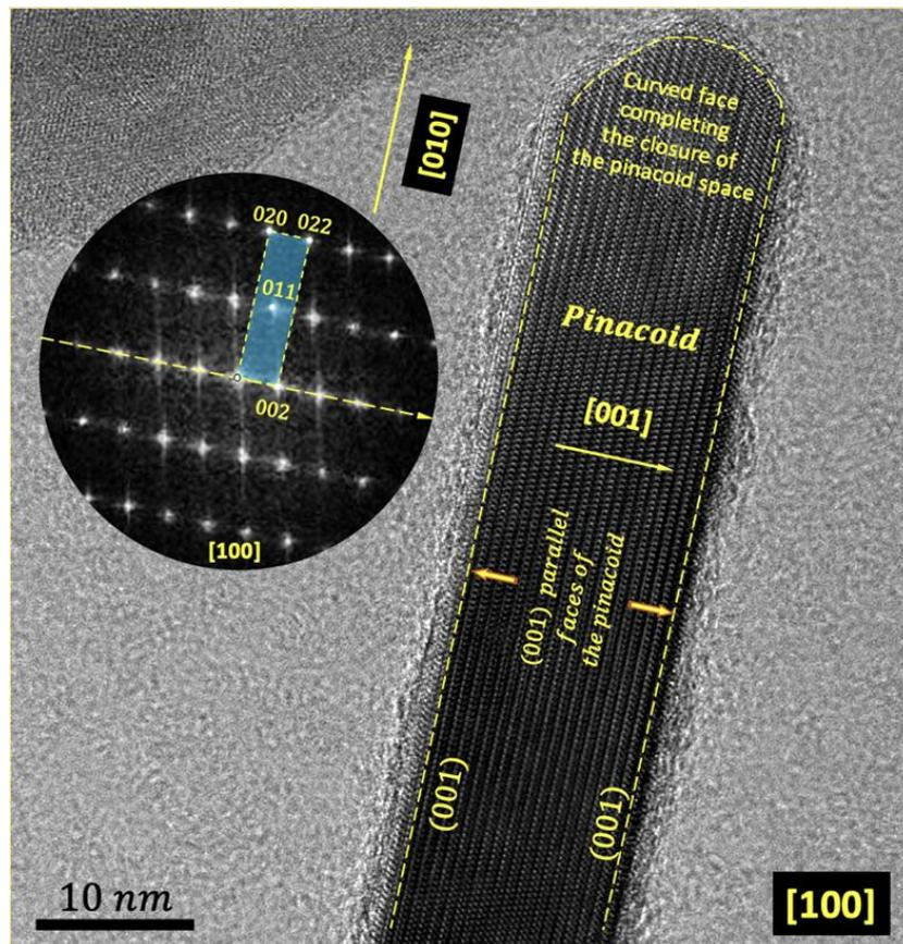
Fig. 3.9: HRTEM image of the BOC nanosheet observed edge-on along the  $[100]$  direction. Corresponding FFT along  $[100]$  zone axis with the centred tetragonal unit cell. One can notice that the edge-on faces of the nanosheet are parallel to  $(001)$  plane as pointed out by the corresponding FFT. This geometric information indicates that we are in the presence of a pinacoid (a pair of parallel faces Supplementary Material S3.3).
