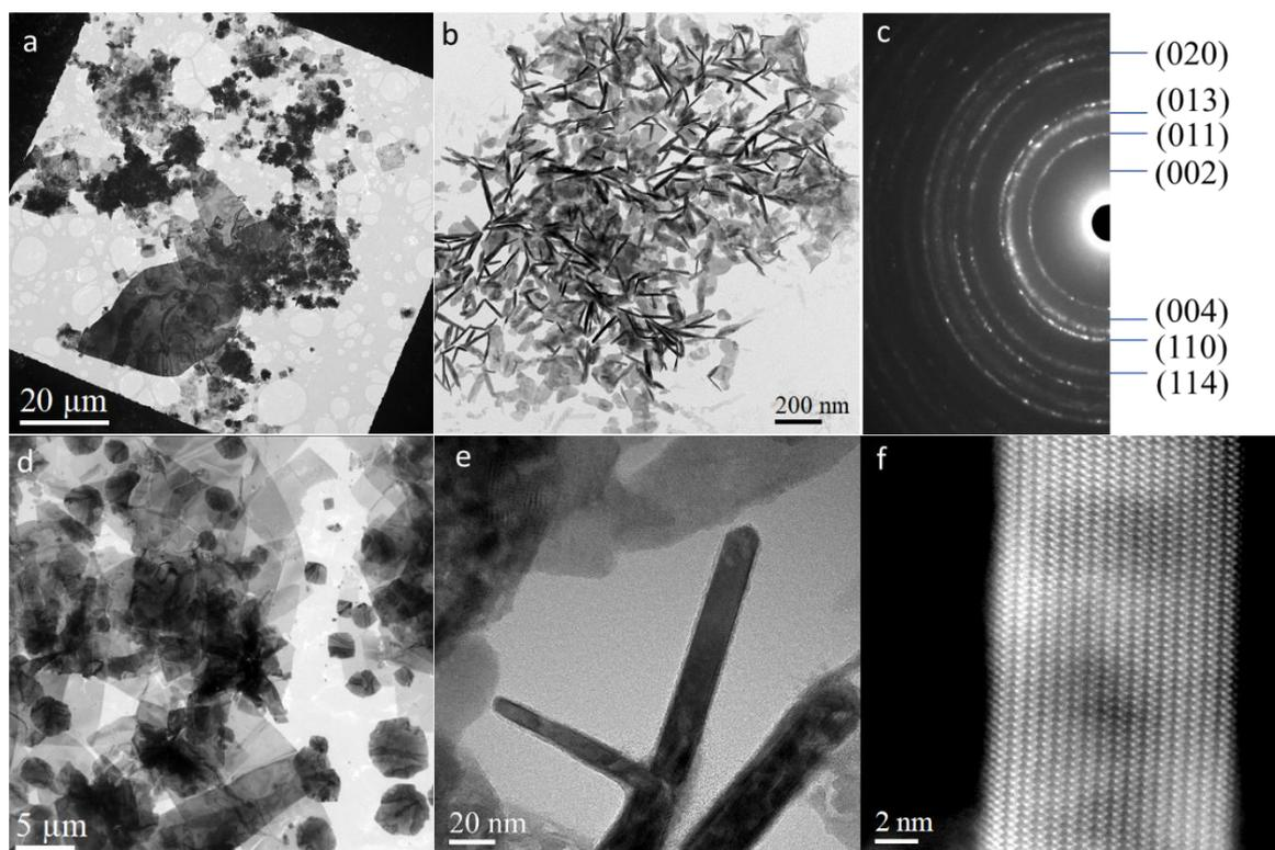
**Supplementary Material S2.2:** Set of nanosheets as in **a)** water and **d)** liquid nitrogen. **b)** Thin rolled nanosheets. **c)** Corresponding diffraction pattern and d-spacings corresponding to  $\text{Bi}_2\text{O}_2\text{CO}_3$  (JCPDS card 41-1488). **e)** High magnification of a properly-oriented cross-section of a nanosheet. **f)** Atomic resolution of the corresponding structure showing the zig-zag structure of  $\text{Bi}_2\text{O}_2\text{CO}_3$ .
