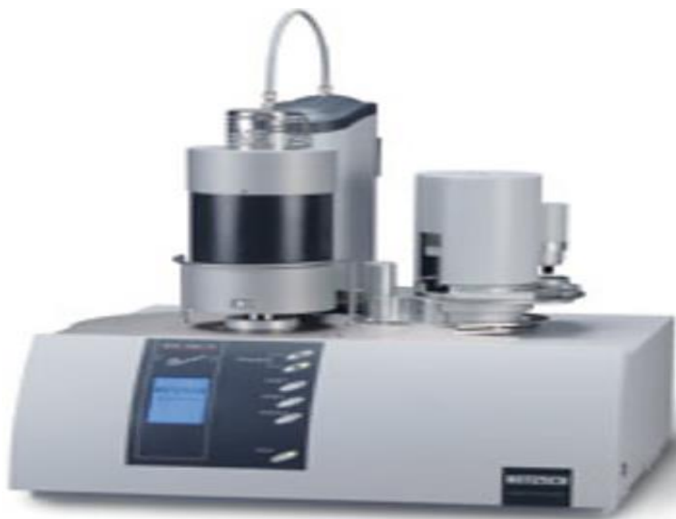
Figure A. 12 : Thermobalance NETZSCH STA 449 F3 Jupiter .
