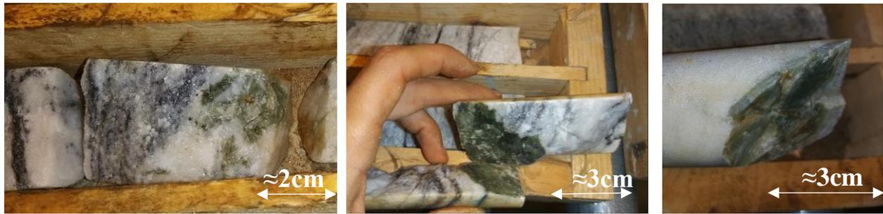
Fig. 3.17. Three photos of talc mineral within Dolomite in the drill cores. On the left, an example of talc minerals within rock matrix. Middle and right photos show talc-filled fractures. Middle one shows a very thin infilling whereas the right figure show an infilling of several millimeters.
