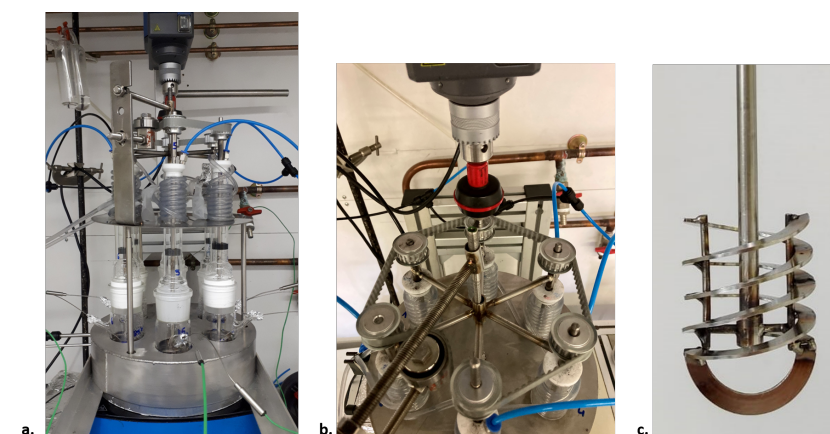
Figure A1. Medium-sized experimental system. (a) Whole system. (b) Pulleys-belt. (c) Mechanical agitator.
