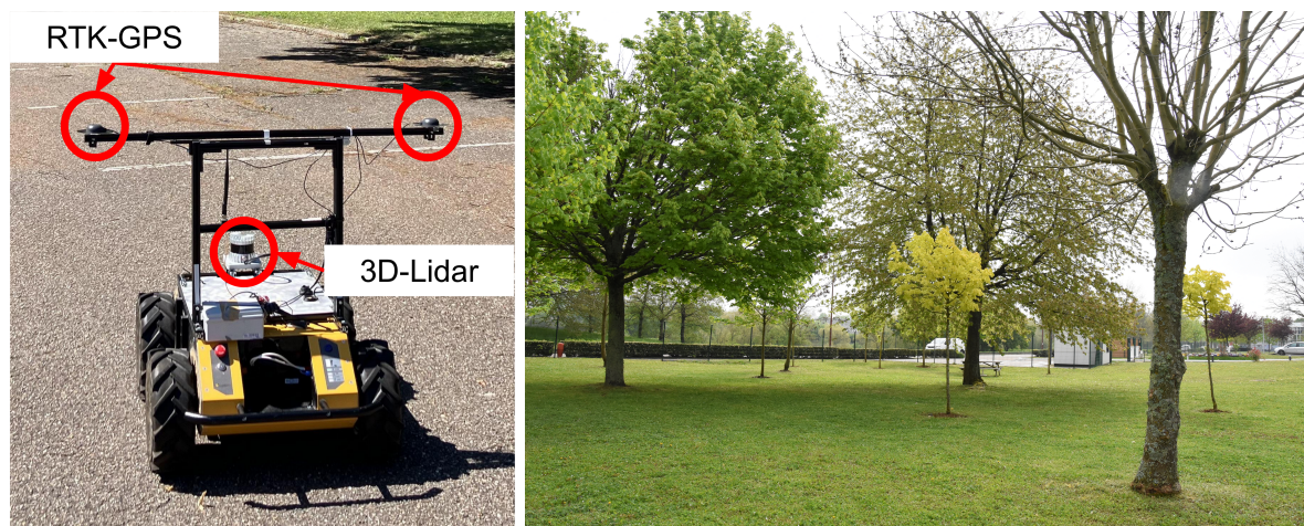
Figure 1.1: The Husky Robot with its sensor suite and the type of environment we consider.
