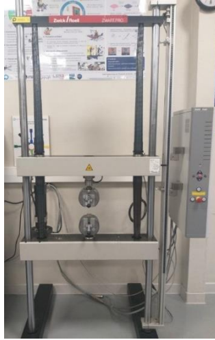
Figure 2.10 Machine de traction uni-axiale Zwick/Roell® (cellule force de 10KN).
