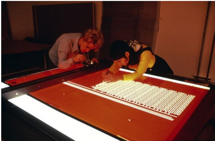
Figure 2.10: Rubylith operators (1970 ca.) from the Computer History Museum website . Copyright Intel Corporation.
