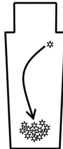
Figure 1.7: Representation of the solid sedimentation causing the negative base segregation. From [20].
